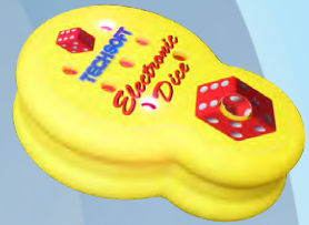
Vinyl stickers on a 3D printed prototype
