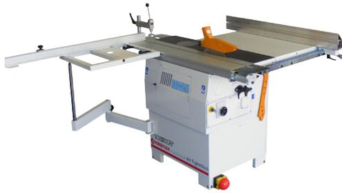
This compact machine will meet most needs for accurate preparation of smaller stock and (with assistance to support the board) will cut any width from a standard 8' x 4' sheet, but will not be suitable for cross-cutting full sheets. If man-made boards can be broken-down first then the sliding table and main rip fence will allow batch preparation of panels up to 700mm in length and/or width.
