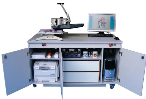
Laser Image Transfer (see pages 118-119) or Sublimation Printing (see page 120-121) requires a PC, printer, heat press and a selection of specialist materials. This workstation has been configured to provide separate key-switch operation of the heat press and printer. The key-switches do not cut power to the PC, so work will not be lost. Secure storage space is included for specialist materials that must not be allowed to become muddled with general print media.
